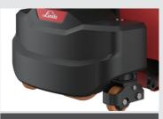
The solid metal driving cover can effectively protect the driving motor in all directions and provide a safety guarantee for the operators at the same time. Both sides are equipped with a castor wheel to reduce shakes and bumpiness caused by uneven road surfaces. It also helps avoid scraping and improve the stability of tall cargo handling.
